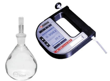
Figure 2.1 Pycnometer and densimeter, devices to measure the density of water.
